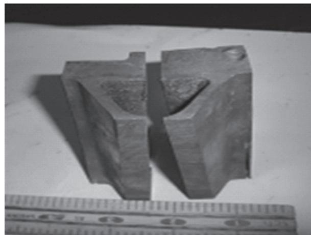
(a) Slicing the cooling channel.
