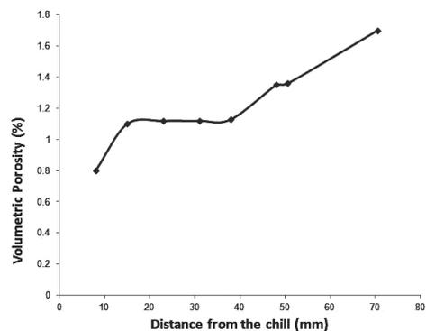
**Fig 1. Relation between distance from the chill and volumetric porosity of as cast Al-Cu alloys**
