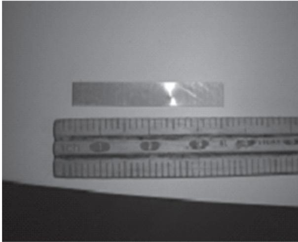
(b) Rectangular strip extracted from cooling channel
