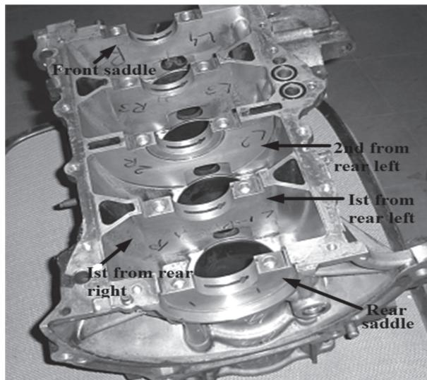
(a) Labeling of the die cast Al engine block
