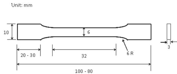
Fig 5. Standard Tensile Specimen
